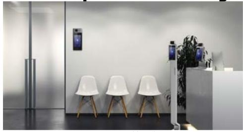
Hikvision's MinMoe terminals employ face recognition and thermographic technologies to make access easier and safer for work areas, record attendance, and simultaneously screen temperatures without requiring employees to touch a terminal or gate. The "touch-free" nature of the terminals is also suitable in high-throughput scenarios for fast temperature screening with access control, such as offices, factories, retail stores, schools, and so
