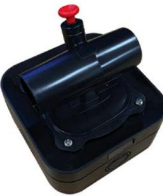
The Vesda Sensepoint XCL – Large Bore from Xtralis is a gas detection solution that utilises the ASD pipe network to deliver superior gas detection via multiple hole (multipoint) sampling. The combined solution provides reliable detection of gases for occupant protection and process monitoring whilst simultaneously ensuring protection against fire threats.
